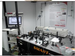
Terahertz imaging system at 0.15 and 0.3THz
