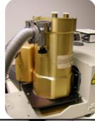
Terahertz time domain spectroscopy system (TDS-THz) range: 0.2-3THz
